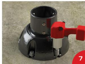
Tighten the concrete screw Anchors in a star pattern, compressing the elastomer and making the base flush to the concrete. Anchor heads must be tightened firmly, flush to base. *Torque Spec: 115 Nm*
