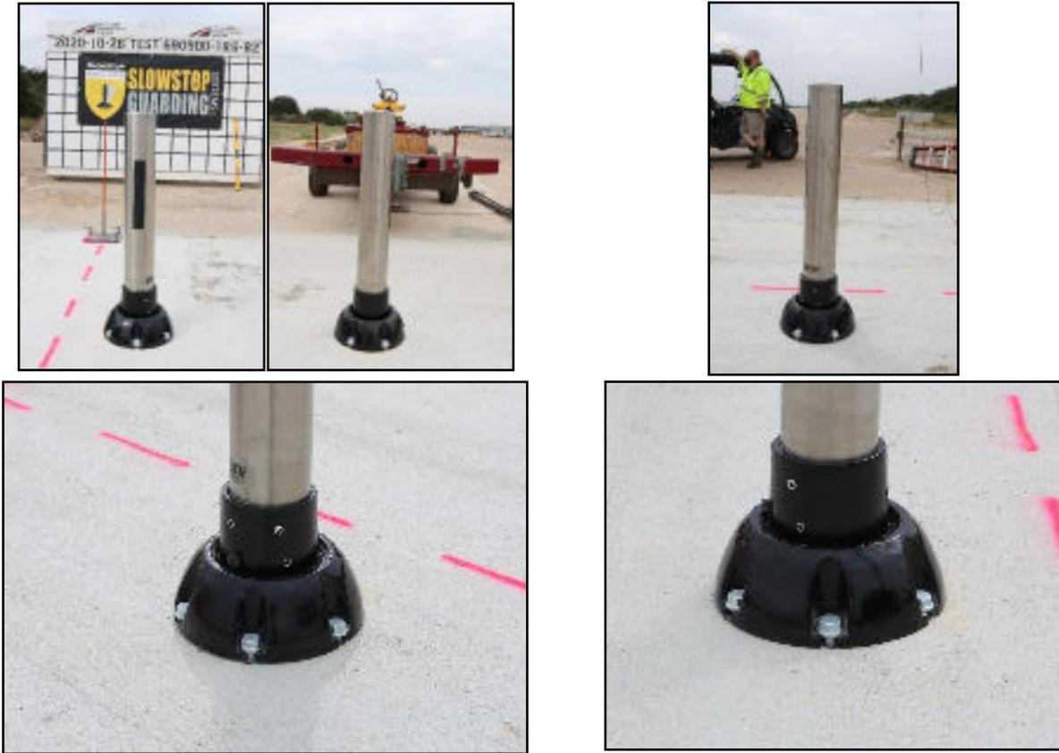
**Figure 3.2. SlowStop® Bollard prior to Testing.**
