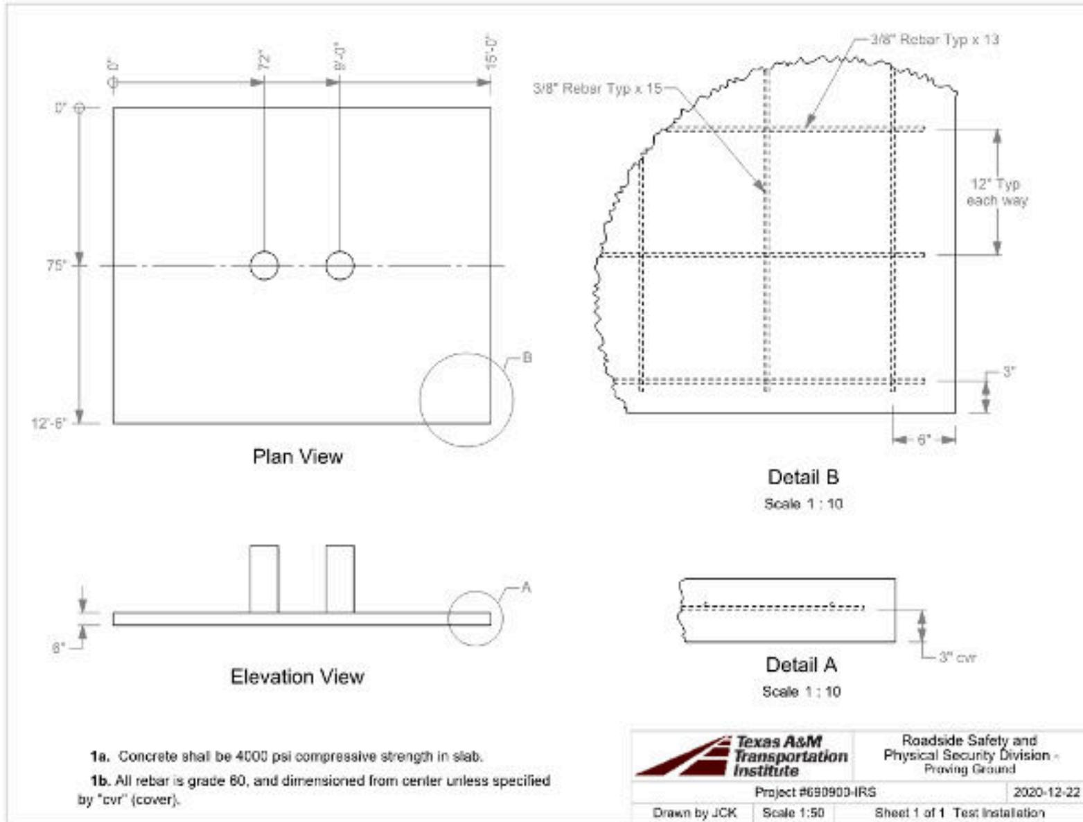
Figure 3.1. General Layout of SlowStop® Bollard.
